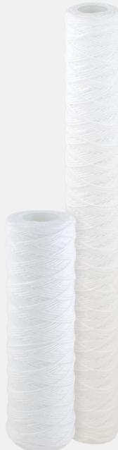
SpiroPure SP-CW series sediment filters are manufactured from polypropylene string-wound filter media. The wound polypropylene string captures and reduces fine sediment, such as sand, rust, silt, and scale particles. The polypropylene cord is wound around a durable polypropylene core for cartridge strength.
