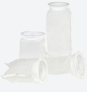
The SP-BN Series of liquid bag filters by SpiroPure are designed to fit any 10 or 20 inch standard bag filter housing for a variety of applications. The nylon monofilament mesh provides increased strength and stretch resistance, giving them a high solid retention and flow rate.
